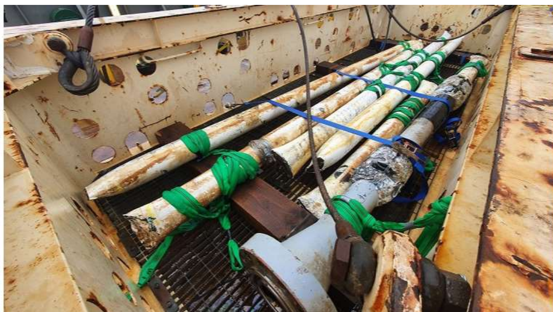
Photo #10 Cut WI flowline end sections recovered in basket
