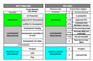
Fig. 1.2 Comparison of NPD and SPE reserves and resources classification systems
